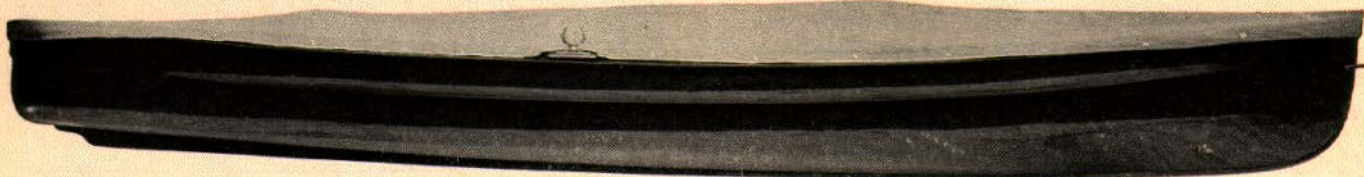
"WATERPROOF CANVAS COVER" shown on Square Stern Spenson Model. Wood bows are bent to shape to hold canvas in position shown in picture. These bows reach across from gunwale to gunwale and are strapped to underside of cover. "Lift-the-Dot" fasteners, as on automobile curtains, secure the covering along sides. Price for Square Stern Spenson Model or Square Stern Model $18.00.
