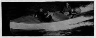
cedar planking is brass screw fastened to oak or ash ribs. Joints are laid in marine compound and tightly compressed to eliminate leaking. Deck, open gunwales, coaming and transom are mahogany. One side stern seat
