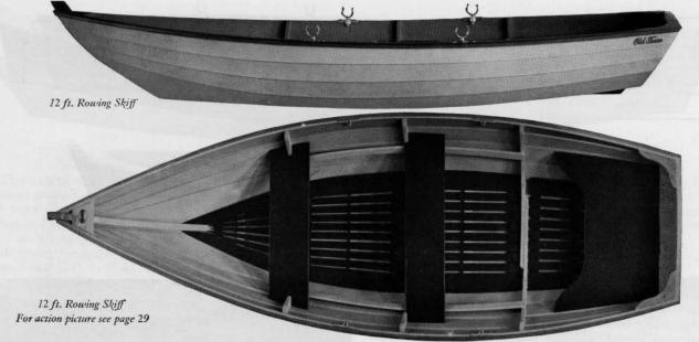
Style of this skiff dates back over ninety years but the design has been successively improved to meet modern requirements. Rugged construction, enduring materials and seaworthy design for sturdy use on ocean, lake, pond, river or stream. Lapstrake construction — sometimes called clinker built. Bottom boards 13/16 in. native pine. Side boards 3/16 in. native pine. Frames, knees
