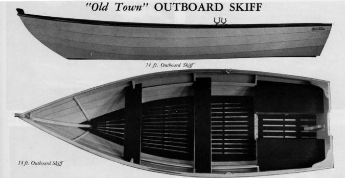
This Outboard Skiff is constructed from the same materials and in the same way and painted the same as the Rowing Skiff (page 27). The boats are staunch and able and are built as light as is consistent with seaworthiness, long life and safety. Motors of 2½ H.P. to 16 H.P. give speeds of 5 miles to 20 miles per
