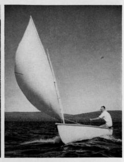
This dinghy is illustrated completely equipped for sailing. The sails are easily removable and after furling will stow inside. Equipped with oarlocks so is usable as rowboat. Stern is strongly braced for outboard motors. Price includes centerboard, rudder with tiller, mast ring and step, 56 ft. area dinghy sail, wire side stays, 24 in. mahogany deck, white color, cotton rope bumper
